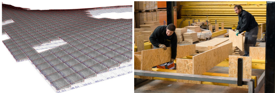
Figure 6: 3d model of formwork table frames; prefabrication of the formwork tables in factory [1]
