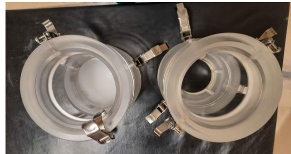
Figure 2: Printed PLA (density of about 1.3 \text{ g cm}^{-3} ) designed filter which has been added to the A10 LIAC. The filter presents a conical shape with 1.3 mm height at the center.
