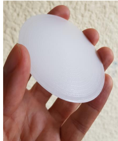
Figure 2: Printed PLA (density of about 1.3 \text{ g cm}^{-3} ) designed filter which has been added to the A10 LIAC. The filter presents a conical shape with 1.3 mm height at the center.
