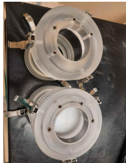
Figure 3: The two upper part of the A10 of the LIAC used in this work. The top image shows the top view of both A10, with the designed filter embedded and the standard one. The bottom image shows the opposite view.
