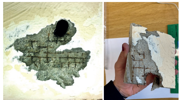
Figure 11 | Sample in the portion of the arch presumably made with Type 680 concrete (on the left), and a sample in the portion of the arch presumably made with Type 500 concrete.
