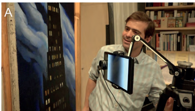
Figure 4 | A) NU-ACCESS faculty affiliate, Professor O. Cossairt, using the iPad deflectometry app developed by NU-ACCESS and the Northwestern's Computational Imaging Lab at the O'Keeffe Museum in Santa Fe, New Mexico. B) Schematic diagram of image capture with structured light for surface metrology.
