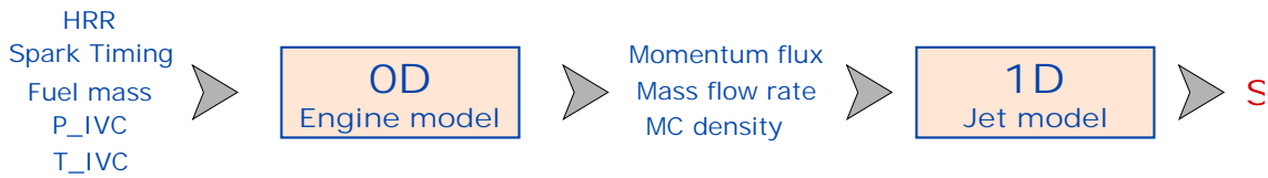
Figure 3: Schematic layout of the modeling workflow coupling a 0-D engine model with the 1-D gas jet model.
