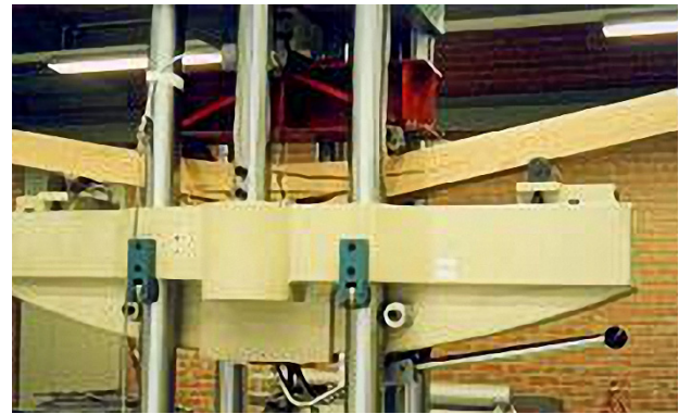
Figure 4 | Sequence of the simple flexion breakout test carried out on a laminated conditioned Quercus cerris beam.
