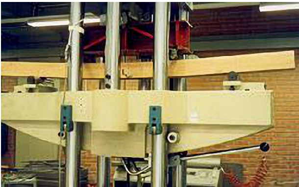
Figure 4 | Sequence of the simple flexion breakout test carried out on a laminated conditioned Quercus cerris beam.
