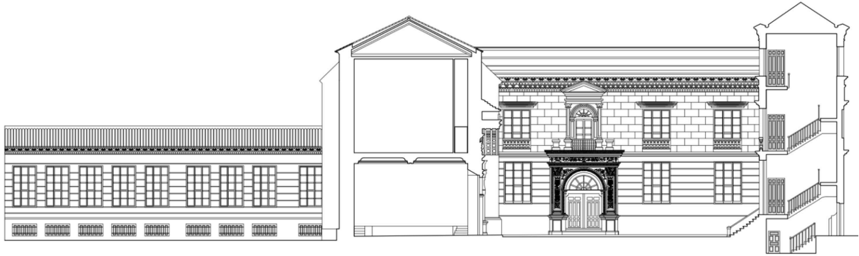
Fig. 17.- Cross-section and elevation of the Institute of Guadalajara. Drawing: Fernando García Román and Eduardo González Muñoz.
