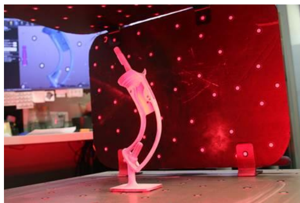
Figure 2: Frame of transitional revolver in the 3D scanner.
