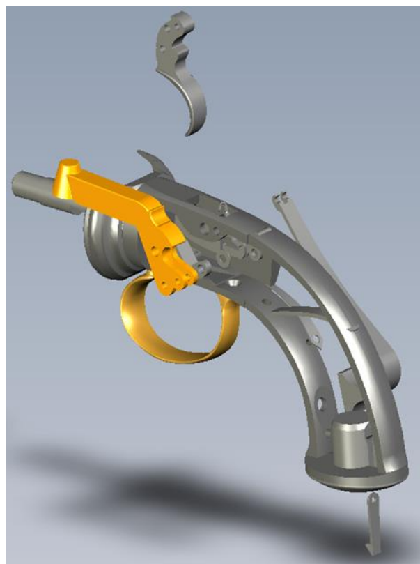
Figure 12: Grip, trigger, hammer, and mainspring of the transitional revolver.
