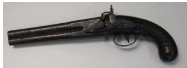
Figure 4: Exterior of the double-barreled pistol, converted from flintlock to percussion cap ignition.
