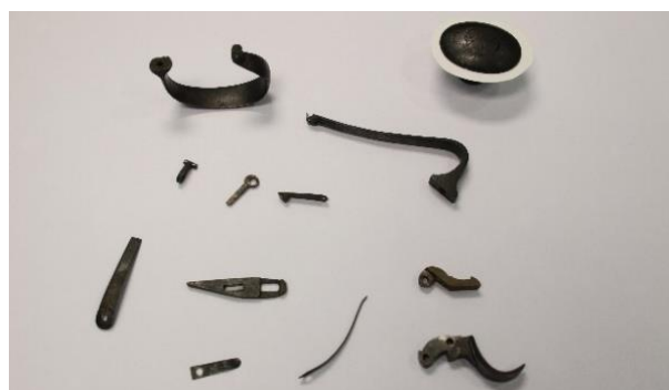
Figure 13: Small metal components from the transitional revolver, including trigger assembly components and leaf spring.
