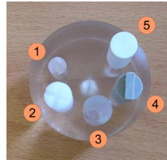
Fig. 2. Phantom with inserts: 1, Air; 2, PTFE; 3, PMMA; 4, PE and 5, POM.
