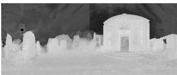
Figure 6: Point cloud of external scans of the church.
